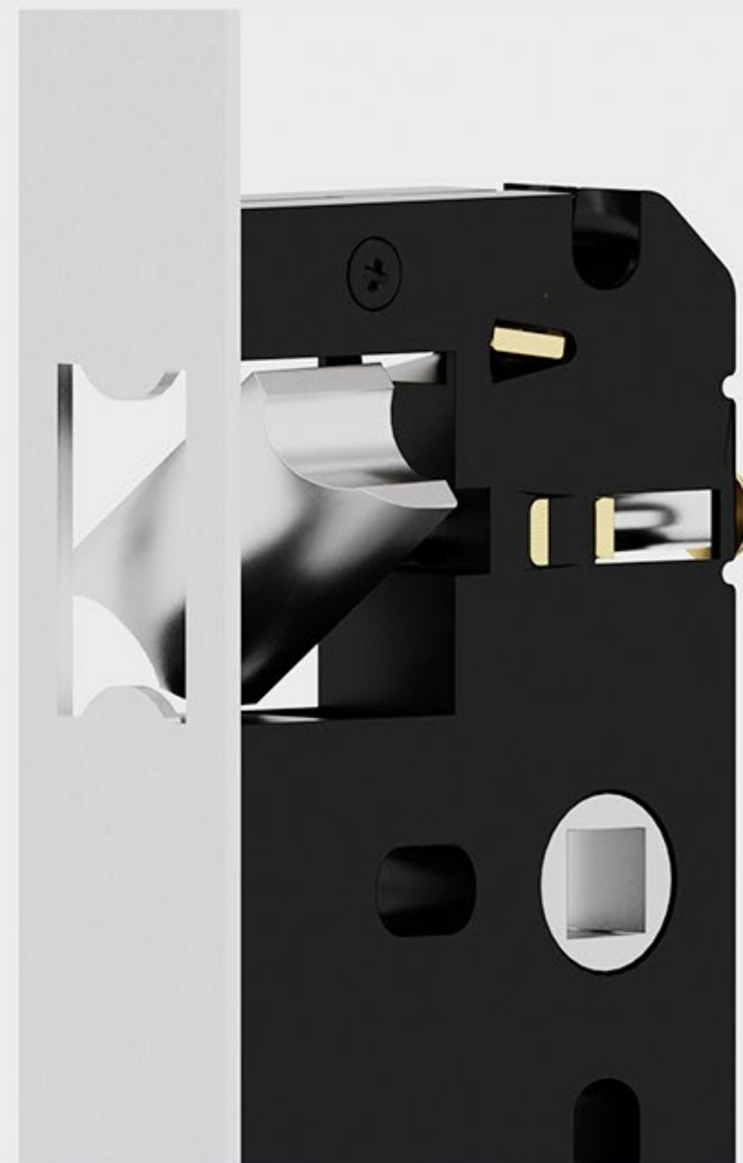
B) TO CHANGE DIRECTION OF LATCH LIFT LEVER, DEPRESS LATCH AND ROTATE 180° INSIDE OF GATE DIRECTION
